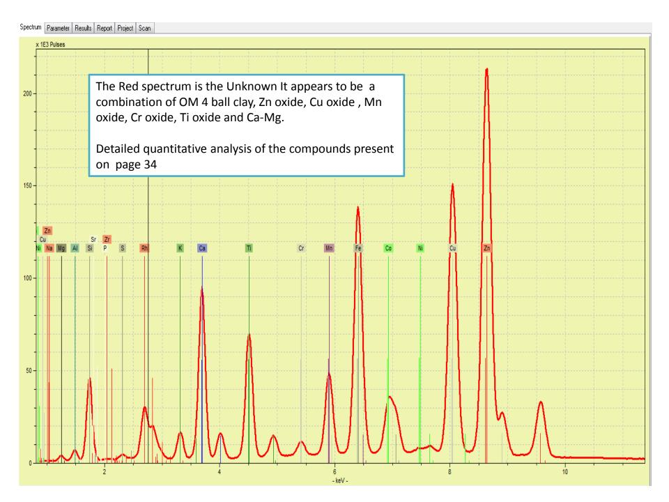
Bruker has software that can quickly give one the net number of photons from each element in a given spectra. This allows one to quickly compare the relative concentration of any element in any material, uniform or non-uniform. One can do up to 50000 spectra at once. The software is called ARTAX. This was done to all the data that was taken on the samples sent. Direction and the result of this analysis follows.
